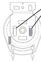
Once hooks are aligned control end will drop into position
