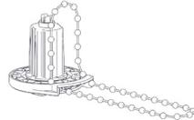
STEP 3 – place 1 ball into tooth and pull chain clockwise
